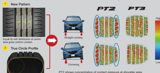
Uniform deflection of sidewall area relaxes concentration of contact pressure at shoulder area when cornering...
